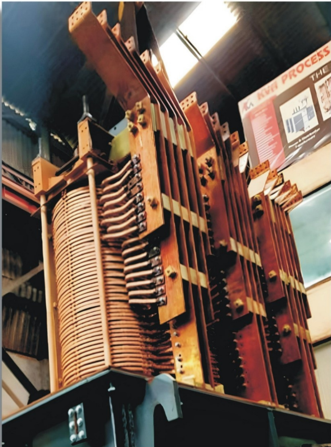
Core & Coil Assembly of Submerged Arc Furnace Transformer
