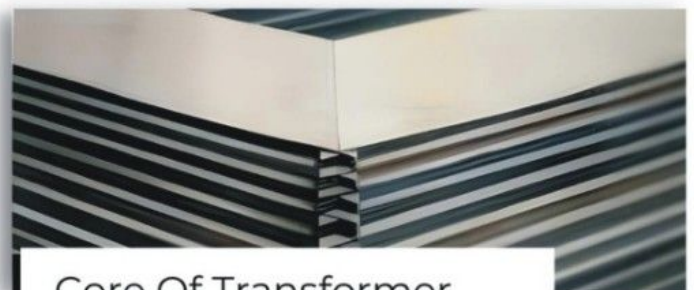
Core Of Transformer
